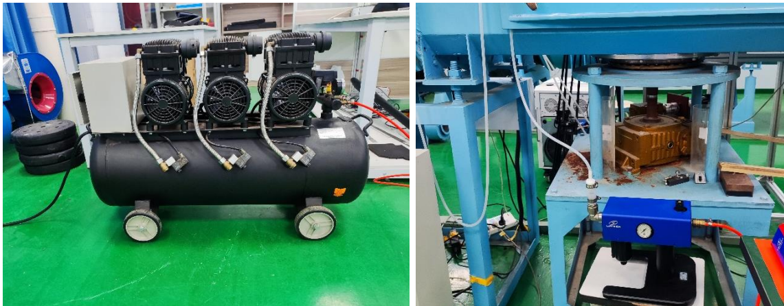
Fig. 2: Compressor and fog generator.
