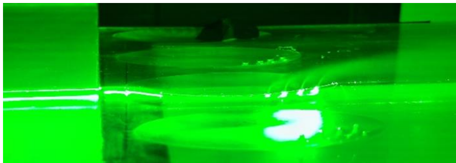
Fig. 7: An experimental model undergoing PIV assessment.
